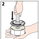
Remove protective cellophane wrapper from filter cartridge and rinse under running water. Remove the Bubble Tube from the inside of the aguarium (if fitted). Offer up filter cartridge to bubble tube and twist the bubble tube in the direction of arrow ensuring all cartridge tabs are fully locked.
