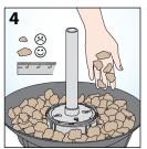
Wash the ceramic media supplied thoroughly before placing around the filter body, ensuring none remains on top of the filter housing.
