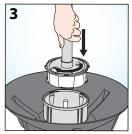
Ensuring no objects are in the way, insert bubble tube and filter cartridge assembled in step 2 into the aquarium and lock into place by giving the bubble tube a quarter turn.
