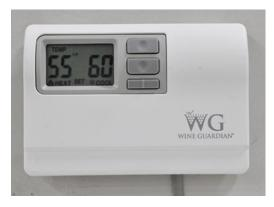
The Wine Guardian remote interface controller is a combination temperature and humidity controller with single stage cooling, heating and humidifier control. Each Wine Guardian unit is supplied with a remote interface controller and 50 feet of communication cable. It is wired at the factory for testing prior to shipment.
