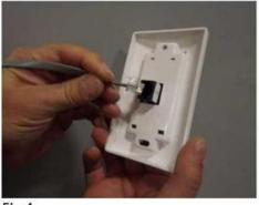
5. Plug in the communication cable to the back of the remote sensor and attach to the wall using the two screws provided in the kit. (Fig. 4)
