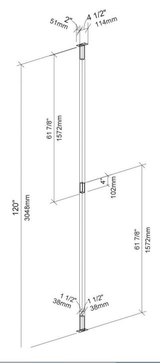
Cut to Fit on Site With Mounting Base extened 2" (51mm), max installation height is 122" (3099mm).
