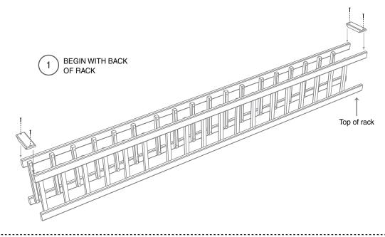
3. Attach the middle standard connectors so that the top edge of the lower connector is 26 5/8" from the bottom of the rack, and the top edge of the upper connector is 51 3/4" from the bottom of the rack. Secure the middle connectors using the screws provided. This is the back of your rack. (figure 2)
