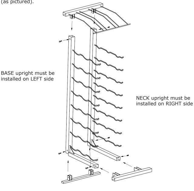
\*Optional: To connect units side-by-side, simply remove the plastic end caps and insert the provided couplers.
