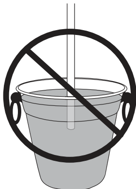
WRONG: Drain line is under water.
