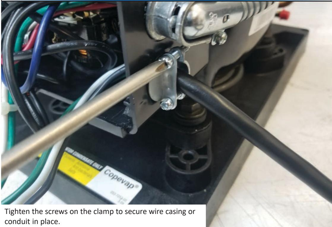
Tighten the screws on the clamp to secure wire casing or conduit in place.
