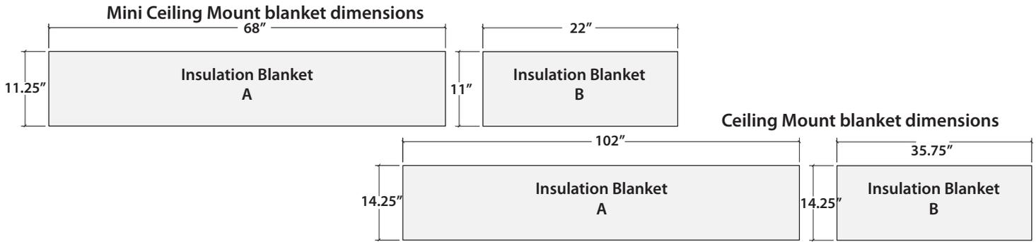
1. Once mounting bracket location has been selected and installed, proceed to the insulation blanket installation.
