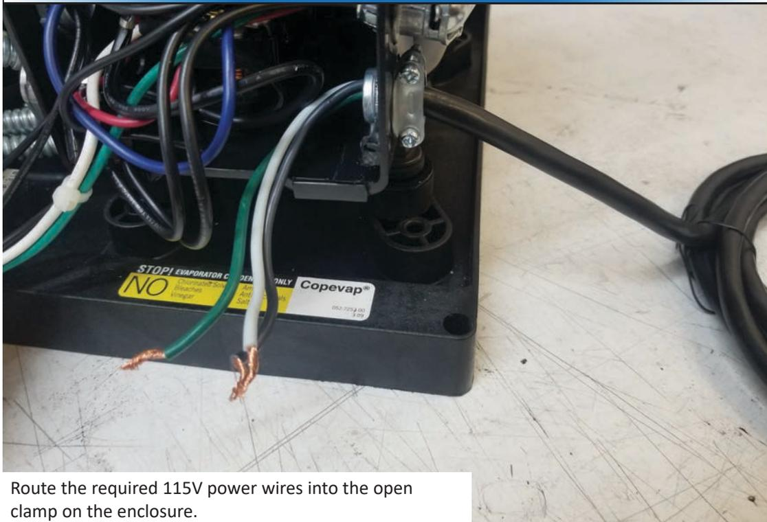
Route the required 115V power wires into the open clamp on the enclosure.
