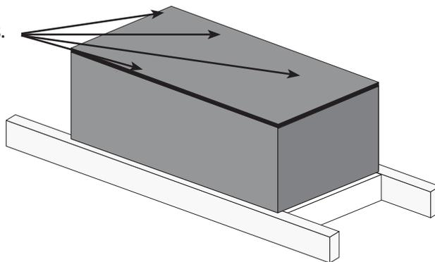
10. Once insulation is installed, apply foil tape to all seams, covering them completely.
