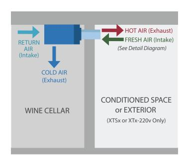
\* The hot air exhaust can be rear or top vented.
