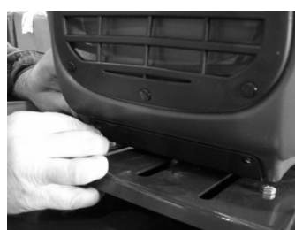
5/ Raise seat adjustment lever & slide seat fully to the rear. Screw the cap head screws into the rear seat inserts by hand & tighten using 5mm A/F Hex Allen Key
