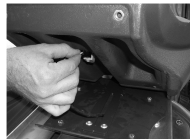
3/ Connect the protruding wires to the seat switch.
