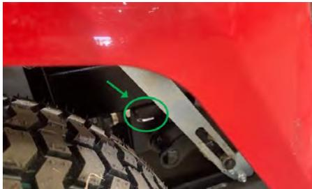
**Stockman Plus & Pro Only:** Transaxle Pump By-Pass Lever is located at the front of the transaxle and near the middle of the chassis. Move lever to back for normal operation or move lever forward for free wheel.
