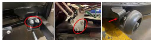
6. Loosen lock nuts on rear linkages.
