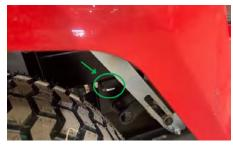
Stockman Plus & Pro Only: Transaxle Pump By-Pass Lever is located at the front of the transaxle and near the middle of the chassis. Move lever to back for normal operation or move lever forward for free wheel.
