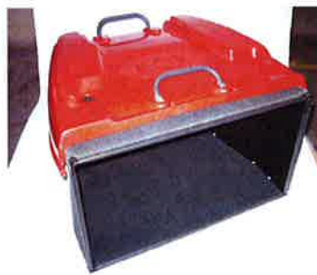
13/ Using the two M8x20 screws and nyloc nuts fit the other handle to the front of the catcher with the handle holes facing forward. Tighten all four handle screws.
