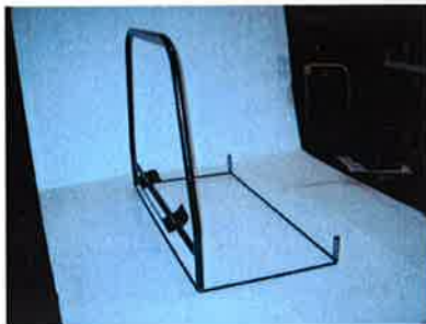
2/ Fit the upper frame over the outward leaning front frame short tubes. Note: The two holes in the upper frame near the bent corners must face inwards.
