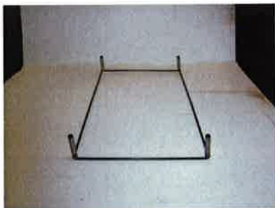
1/ Clean tubes with emery paper. Place the front frame with the short tubes in each corner on a flat surface with the short tubes up.
