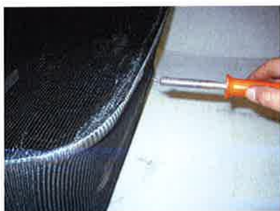
10/ Using a small soldering iron melt through the mesh at the four bolt holes in the upper frame to suit the handle bolts.
