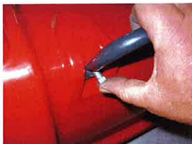
10/ Using a small soldering iron melt through the mesh at the four bolt holes in the upper frame to suit the handle bolts.
