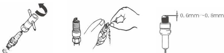
(1) Remove ignition plug (2) Clear off carbon deposit (3) Adjust clearance.
