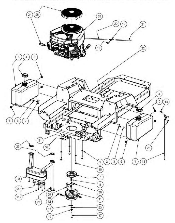
ENGINE ANCILLARY COMPONENTS 22&24HP B&S RECTANGULAR MUFFLER TO SUIT 42" MOWING ATTACHMENT
