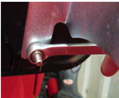
Attach nuts to the front studs
