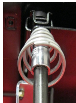
Attach conical springs, washers & nuts to the rear studs
