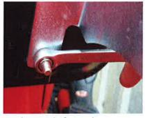
Attach nuts to the front studs
