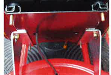
Locate studs of the seat assembly runners through the seat mount
