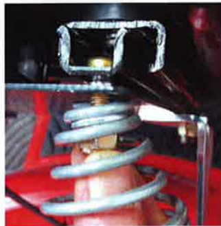
Attach conical springs, washers & nuts to the rear studs
