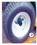
Cast Alloy Rim Use AM305 Rim TT650X8 Tyre & Tube STU650X8 Tube 14001 Hub, Adaptor SH1025M Bolt (3) W061216 Washer (3)
