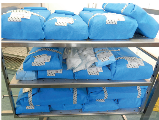
Insufficient space between packs and loaded unevenly – sterilizing agent cannot permeate around the packs.
