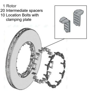
To fit the OEM Rotor it is placed over the hub and the intermediate spacers are placed either side of the hub location splines until all 20 are fitted and the disc is secure. Then the 10 location bolts are fixed into place.
