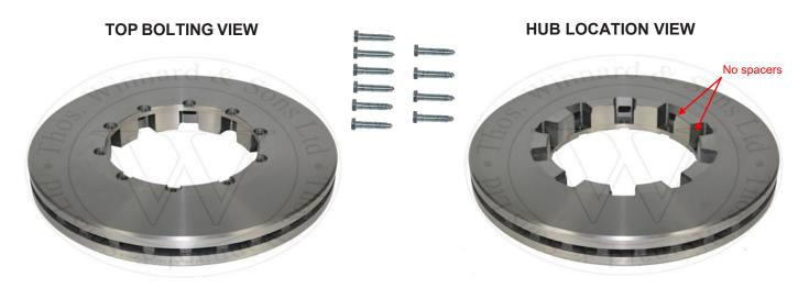
To fit the Winnard rotor simply present the rotor over the cleaned hub location splines and press into place. Fit the hub location bolts and torque up to 24Nm +/-2.
