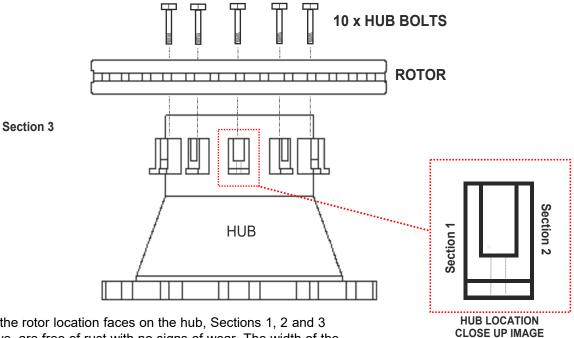
1. Make sure all the rotor location faces on the hub, Sections 1, 2 and 3 illustrated above, are free of rust with no signs of wear. The width of the spline location, section 3 on the image, should be measured, the new width is 1.1811" (30mm) the maximum allowable wear is 0.015" (0.381mm).
