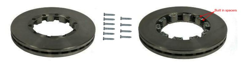
To fit the Winnard rotor simply present the rotor over the cleaned hub location splines and press into place. Fit the hub location bolts and torque up to 24Nm +/-2.
