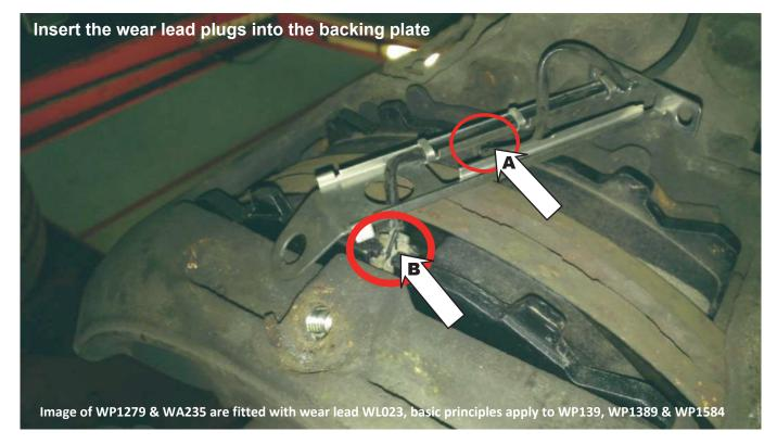
PLEASE NOTE: THE WEAR LEAD PLATES SITS ON TOP OF THE RETAINING SPRINGS - NOT UNDERNEATH.
