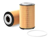
Length / Overall Height193.50 mmMedia TypeCelluloseLength193.90 mmLargest End ID52.50 mm
