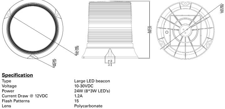
Current Draw @ 12VDC Flash Patterns Lens Base Flying Leads IP Rating Operating Temperature Weight Dimensions Approvals 10-30VDC 24W (8\*3W LED's) 1.2A 15 Polycarbonate ABS 350mm IP66 -20°C to +50°C 0.550Kg 16.3cm D x 16.76cm H CE, ECE R65 (Single Flash:120 fpm Pattern no.3)
