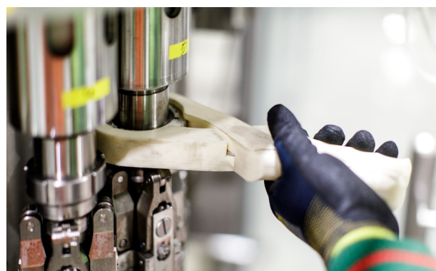
3D printed tools make maintenance easier and less time consuming
