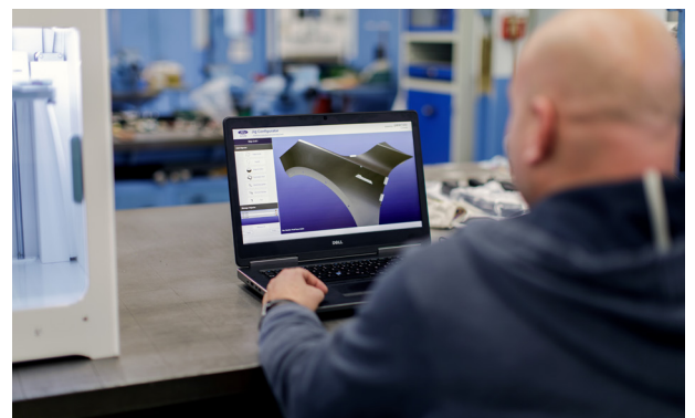
Trinkle's software enables workers to generate tools which can be directly sent to the Ultimaker 3D printer
