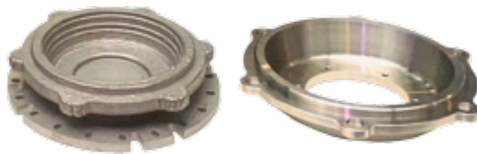
Wheel set bearing cover. 3D printed net shape (left) and post-machined part (right) [Source: Deutsche Bahn]
