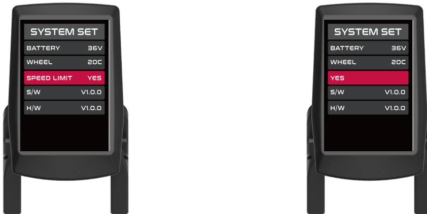
Figure7-9: Speed limit setting interface
