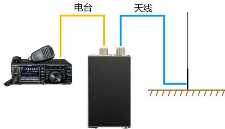
Radio - Antenna - Antenna feeder connection
