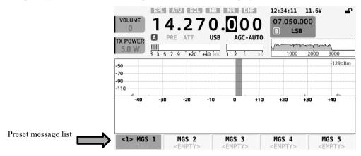
X6100 can pre-store 5 preset messages. These messages can be used for automatic transmission of CW, RTTY and BPSK. Click any MGS label to enter the editing interface, as shown below:
