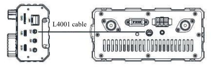
After the X6100 connects with XPA125B power amplifier and antenna tuner AIO through the L4001 cables, the output power can be expanded to 100W.
