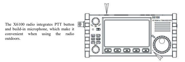
1. Press the PTT button on the top of the device and speak to the built-in microphone hole at the left of large knob to transmit voice.
