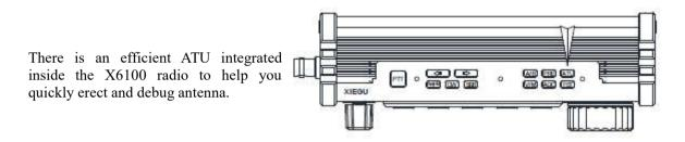
1. Short press [ATU] button to connect with built-in antenna tuner. There will be an antenna icon at the top of screen.
