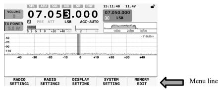
Short press the key corresponding to [RADIO SETTING 1] to enter the "General setting 1" submenu, as shown in the following figure:
