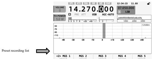
X6100 can pre-store 5 voice messages. These messages can be used for automatic transmission of voice mode. Click any MGS label to enter the editing interface, as shown below:
