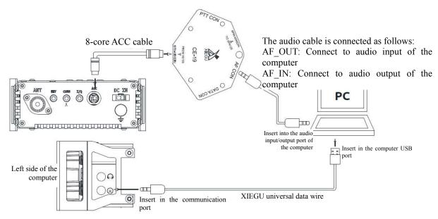
Fig. 1 G90 and Computer Connection Data Communication Diagram
