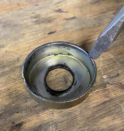
• \*\*Shaving these down will allow the stud of the tie rod end to seat deeper into the tapered hole in the knuckle.
