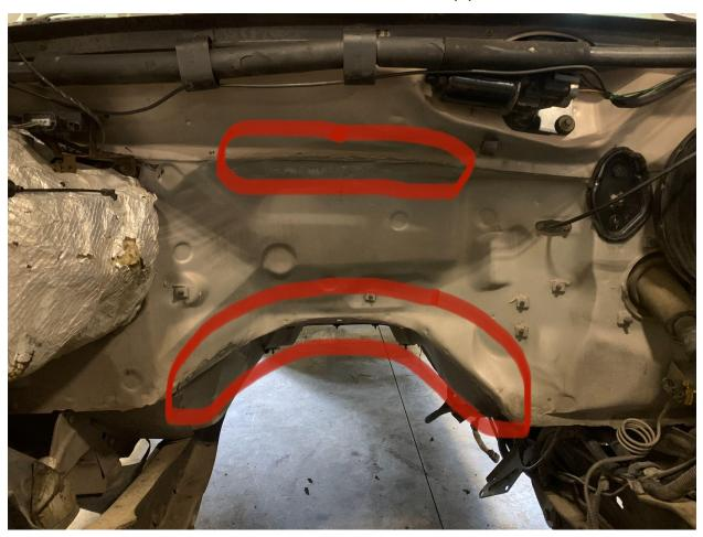
3. Install the frame plates. The frame plate with 4 bolts goes on the passenger side. The frame plate with 2 bolts goes on the drivers side.
