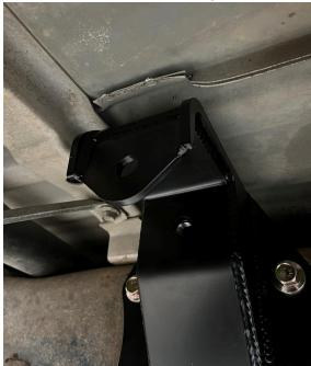
14. Mount the new front leaf spring hanger. The rear holes of the new hanger will bolt into the forward 3 factory holes and the bottom hole will line up with a factory hole in the frame. Then drill the 3 forward holes using the new hanger as a template.
