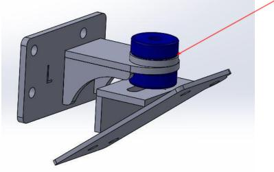
Test fit mounts and make any needed adjustments. Note: Install bushing spacer on top of upper mount. If more clearance is desired between
