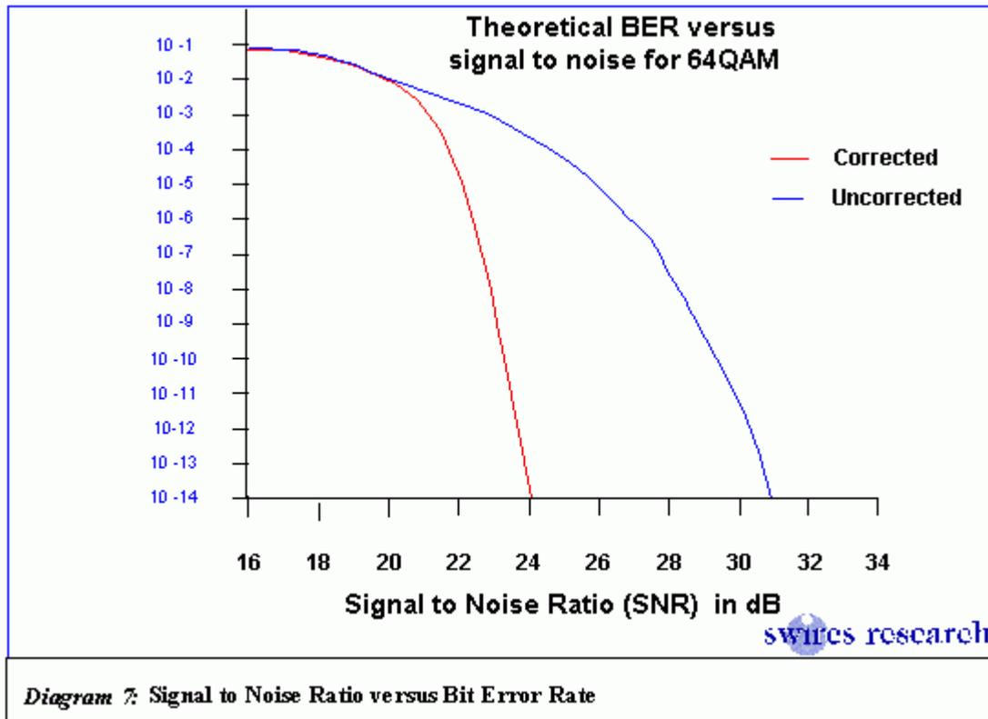
Diagram 7: Signal to Noise Ratio versus Bit Error Rate
