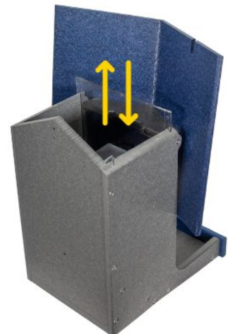
Roof hinges fully open to allow removal of the acrylic seed shield, which also houses the camera.
