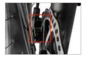
Carefully lift the front of the bike and lower the fork onto the wheel so that the brake rotor enters the caliper, between the brake pads, and the axle enters the fork dropouts fully.
