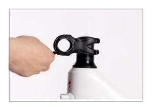
Use the Allen wrench to unscrew the four screws on the face plate.
