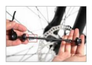
2. Put the quick release screw through the front wheel. Ensure both cone springs point inward. Keep the lever open and thread on the thumb nut a couple of turns. Hold the quick release screw in line with the axle and tighten the thumb nut until the lever can stay parallel to the floor without being held.
