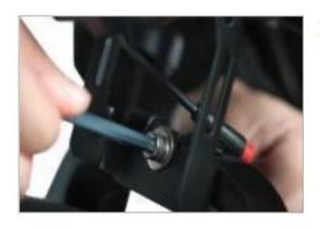
Install the fender/headlight mounting hardware through the headlight bracket, fender, and fork thread in the bolt to attach the fender mounting bracket to the mounting point on the back of the fork, then tighten securely.
