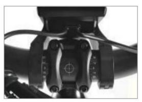
Center the handlebar and tighten the four handlebar stem faceplate bolts evenly and part way.
