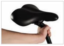
3. Adujst the seat and the head of the seat is parallel with the top tube.
