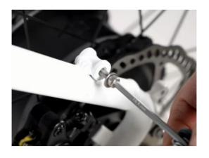
Unscrew the four screws on the rear frame.
