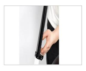
Move the seat up and down by sliding the seatpost in or out of the seat tube. DO NOT raise the seatpost beyond the minimum insertion marking etched into the seatpost tube.
