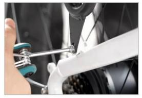
Align the rear rack with the holes and tighten the four screws.
