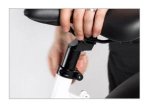
Untighten the quick release lever by swinging the lever open and outward fully.
