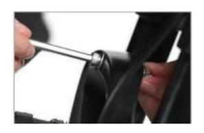
1. Unscrew the corresponding screws on the front fork.
