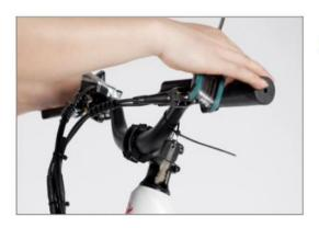
Adjust the handlebar to a position perpendicular to the front wheel and tighten the screws on the stem.
