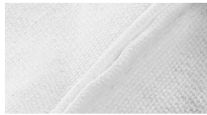
ECRASÉE / CRUSHED SEAM
