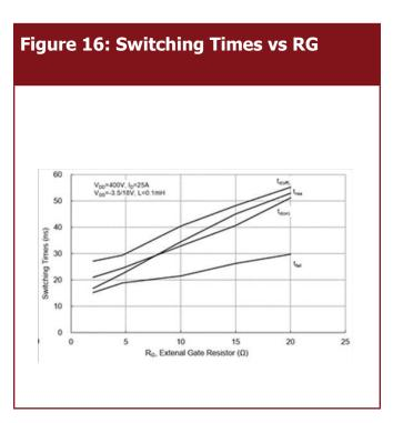
Silicon Carbide (SiC), MOSFET – SiC, 31mohm, 650V, M2
