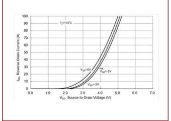
Silicon Carbide (SiC), MOSFET - SiC, 31mohm, 650V, M2
