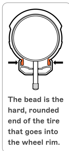
Visually inspect the sides of the tires, using the lines and markings on it as a reference to ensure the bead is inserted into the rim fully and evenly.
