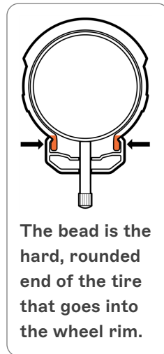
Visually inspect the sides of the tires, using the lines and markings on it as a reference to ensure the bead is inserted into the rim fully and evenly.
