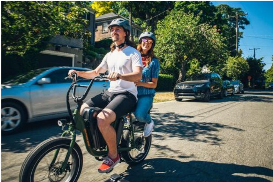
Exclusive 20-inch by 3.3-inch wide multi-terrain tires provide urban comfort and off-road stability. The semi-fat tires are custom-made by the worldwide leader of bike tires, Kenda, in their first one-off creation for a single brand. “We needed a completely new tire to support the different functions of the RadRunner,” said Radenbaugh. “The tires have an extra ply of material and higher load rating than a standard bike tire, plus a built in tire liner and reflective sidewall striping.”
