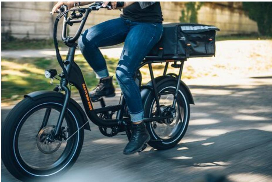
Their eighth model, the RadRunner retains a number of tried and tested features from Rad Power Bikes' lineup, including a powerful geared hub motor (750W in U.S., 500W in Canada, and 250W in Europe), long-range 48V 14 Ah Lithium-Ion battery for 25-45 miles of range per charge, and integrated headlight, taillight, and brakelight.
