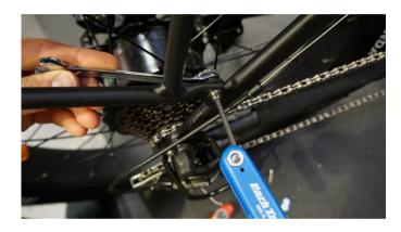
Step 4: Tighten the sliding clamp bolts on the top of the rack to complete the installation.
