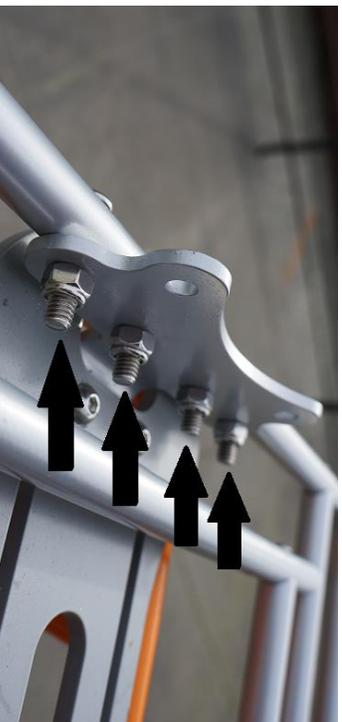
**Step 4:** Securely fasten all button head cap screws holding the tubular structure together. Tighten to 10NM using 4mm Allen wrench.
