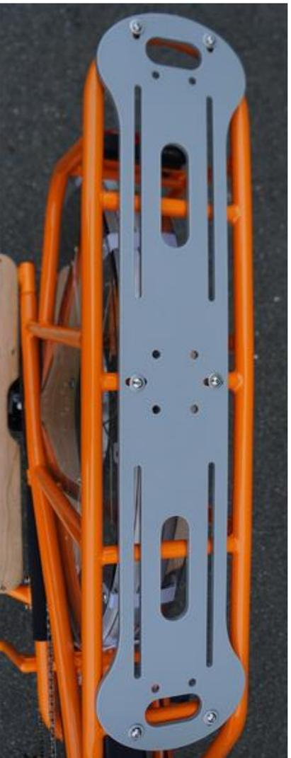
**Step 2:** Once the Caboose is removed from packaging, remove the two end brackets and install as shown by rotating the mounting brackets into the large oval cutouts in the accessory deck on each end. Once inserted and the tab is beneath the deck, secure the bracket to the accessory deck using the provided hardware. Secure to 14 NM using a 3/16" Allen wrench and 1/2" wrench.
