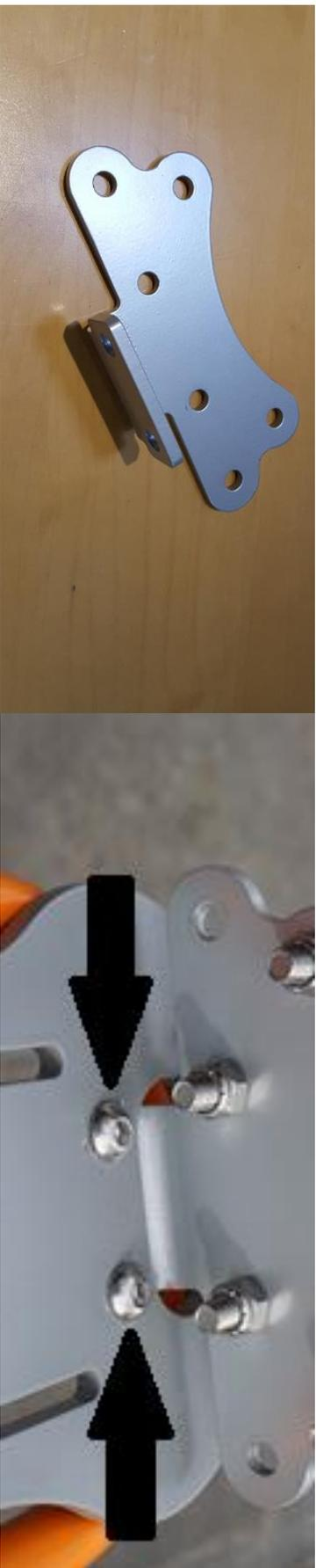
**Step 3:** Fasten all 4 bolts attaching the Caboose tubes to the bracket as shown. Tighten to 14NM using 3/16" Allen wrench and 1/2" wrench as shown.
