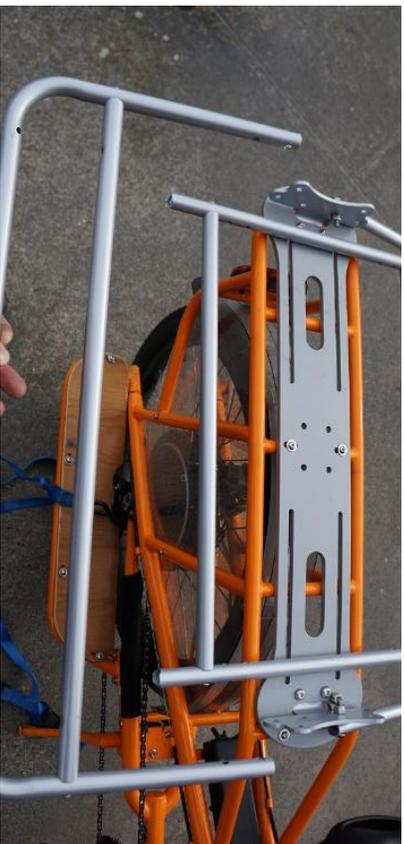
**Step 2:** Raise the tubes up into a V shape as shown below, and attach to the brackets using the 4 holes on each end bracket. Loosely tighten these 4 bolts.
