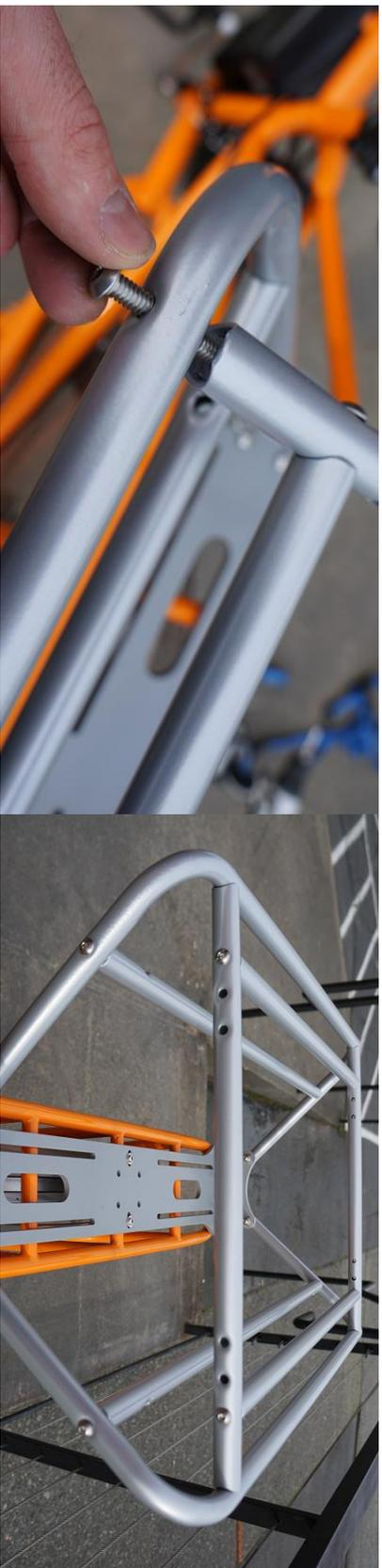
**Step 4:** Set the adjustable center tubes to desired width (7.9", 9.5", and 11.5") using the 3 holes on each end. If you are utilizing a Yepp child seat, mounted to the accessory deck, you will need to remove the two inner most tubes to allow room for the seat.
