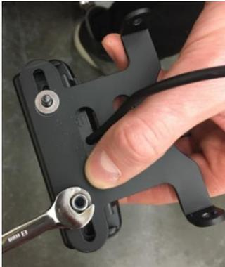
8. **Attach the tail light to the rack mount.** Place the tail light in position on the tail light mounting plate on the rear rack. Install the washers and thread the lock nuts onto the bolt ends by hand. Use an 8 mm wrench to tighten the lock nuts and attach the light securely.
