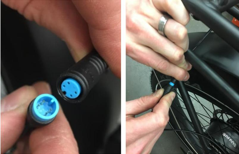
10. **Secure the cable extension to the rack.** Align the cable extension with the cable guides along the rear rack. Keep the cable taut enough to remain clear of the rear wheel spokes, but not so tight the cable could be damaged by over-stretching. Starting near the tail light at the back of the rack, use zip ties to attach the cable to the rack. Working towards the seat post, attach the cable to the cable guides securely using zip ties. Use a flat side cutter to snip off zip tie excess.
