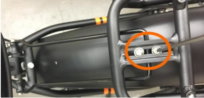
7. **Remove the tail light from the mount.** Use an 8 mm wrench to remove the two lock nuts and washers holding the tail light to the light mount. Set aside for reinstallation.
