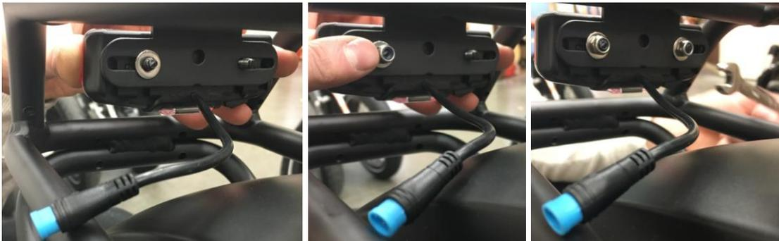
9. **Connect the cable extension to the tail light.** Locate the appropriate end of the tail light cable extension, align the notches and pins, and press the two sides of the connector together without twisting to fully seat the connection.
