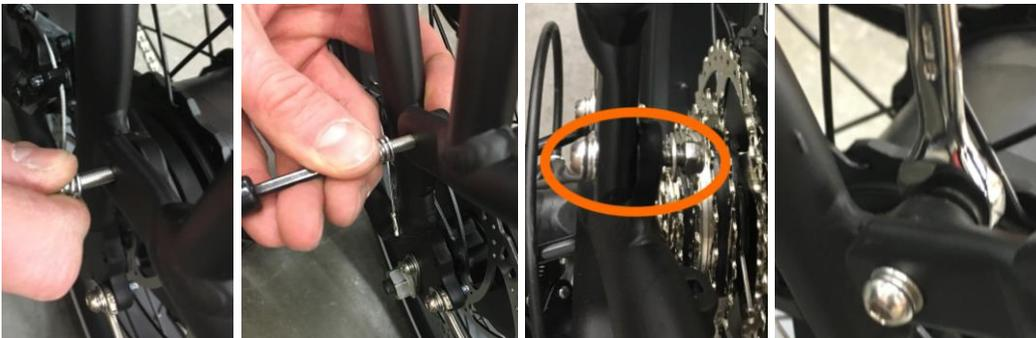
6. **Adjust the rack to be level** by using a 4 mm Allen wrench to loosen the two bolts on the upper mounting arm clamp. Once loose, slide the rack forwards or backwards to adjust the rack angle. To secure, torque the mounting arm clamp bolts to 7 Nm.
