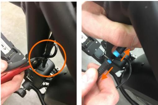
3. **Remove the tail light mounting bracket.** Use a 4 mm Allen wrench to remove both bolts. Set the bracket/tail light and the bolts aside.
