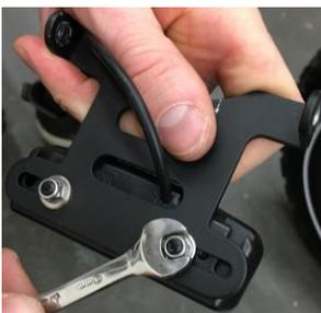
7. **Attach the tail light to the rack mount.** Place the tail light in position on the tail light mounting plate on the rear rack. Install the washers and thread the lock nuts onto the bolt ends by hand. Use a 10 mm wrench to tighten the lock nuts and attach the light securely.
