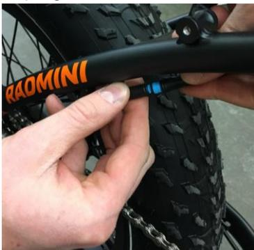
3. **Remove the tail light mounting bracket.** Use a 5 mm Allen wrench to remove both bolts. Set the bracket/tail light aside.
