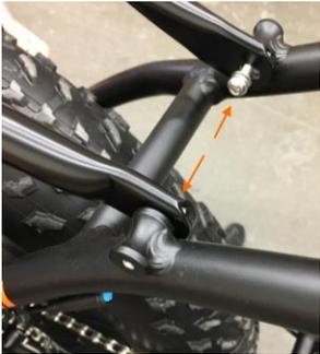
5. **Attach the lower mounting points.** Thread the two remaining (33 mm long) bolts into the mounting point on the rack and then the frame carefully by hand. Use a 5 mm Allen wrench to torque to 7 Nm. Once the bolts are tight against the rear rack lower, install a washer and then thread a lock nut onto the bolt end. Use a 10 mm wrench to torque the lock nut to 7 Nm.
