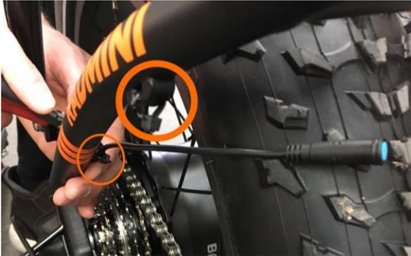
9. **Connect the tail light.** First, ensure the tail light cable runs from the chainstay, outside the derailleur bash guard, and along the inside of the rear rack. Fully seat the connection by aligning the notches and pins on the inside of the connector, and the arrows on the outside, and pressing the two sides of the connector together without twisting.
