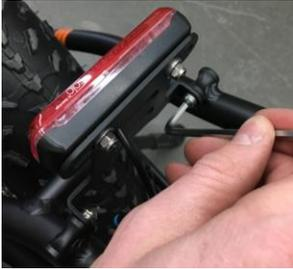
4. **Attach the upper mounting points.** Place the rack in position and attach the upper and lower mounting points using the shorter, 28 mm long bolts. Thread each bolt into the mounting point on the rack and then the frame carefully by hand. Use a 5 mm Allen wrench to torque to 7 Nm.
