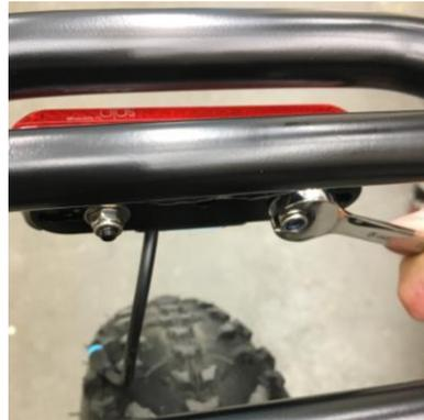
8. **Snip the two zip ties holding the tail light cable onto the seatstay** taking care to not damage the cable housing or wires.
