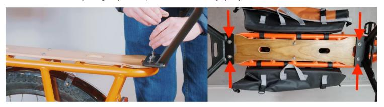
Step 3: Set the adjustable center tubes to desired width using the holes on the cross bars on the front and back of the caboose. If you are utilizing 1 or 2 Yepp Maxi Easy Fit child seat(s) with the Caboose, you will need to move the two inner most tubes to the "L" section to allow room for the seat(s). The L section is the widest section.
