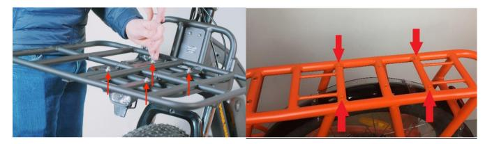
Step 2: Torque all 4 bolts to 3-5 Nm
