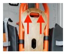
Step 3: Securely fasten both screws attaching the DeckHand to the frame of the RadWagonas shown. Tighten to 3-5 Nm using a 3 mm Allen wrench.
