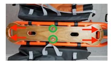
Step 2: To install the caboose on top of the wood deck, use the longer M5x35 mm screws included with the caboose. To install the caboose directly to the rear rack, without the wood deck, use the shorter M5x20 mm screws included with the caboose.
