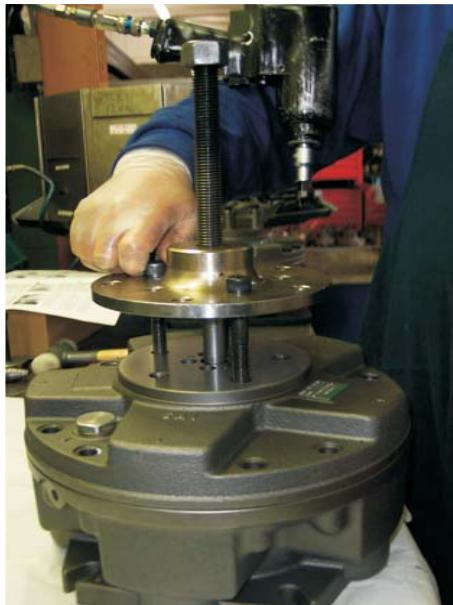
**REMOVAL OF THE RETAINING RINGS OF THE COVER SIDE**
