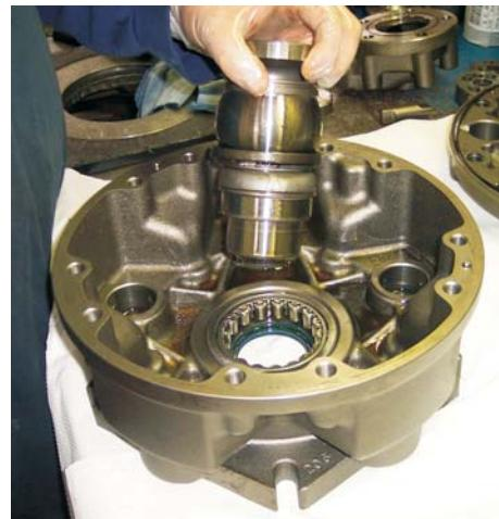
**SHAFT SEAL RING REMOVAL**
