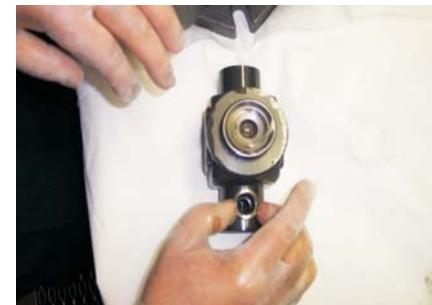
Insert the cylinders into the motor body, putting the plain Trunnions (non seal end) in place. Extend the pistons to bring them in contact with the eccentric, using a suitable tool.
