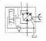
Servo Motor with Shuttle
