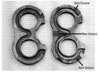
This new wear plate enables better pressure clamping with aerated oil in pumps 1.37 cubic inch or smaller. Aerated oil may occur during a cold start-up in applications with long suction lines or when the mouth of the inlet line is temporarily exposed to air.
