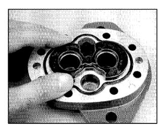
**11** Remove *back-up gasket and seal* from wear plate by extracting with a o-ring tool.
