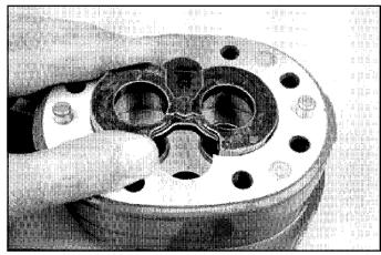
**6** Dip *gear assemblies* into oil and slip into front plate bushings and gears into pockets of body.
