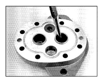
**14** Removing the *plug* in front plate is not necessary, unless you intend to change rotation. See Reversibility - Changing Input Rotation of Pump.
